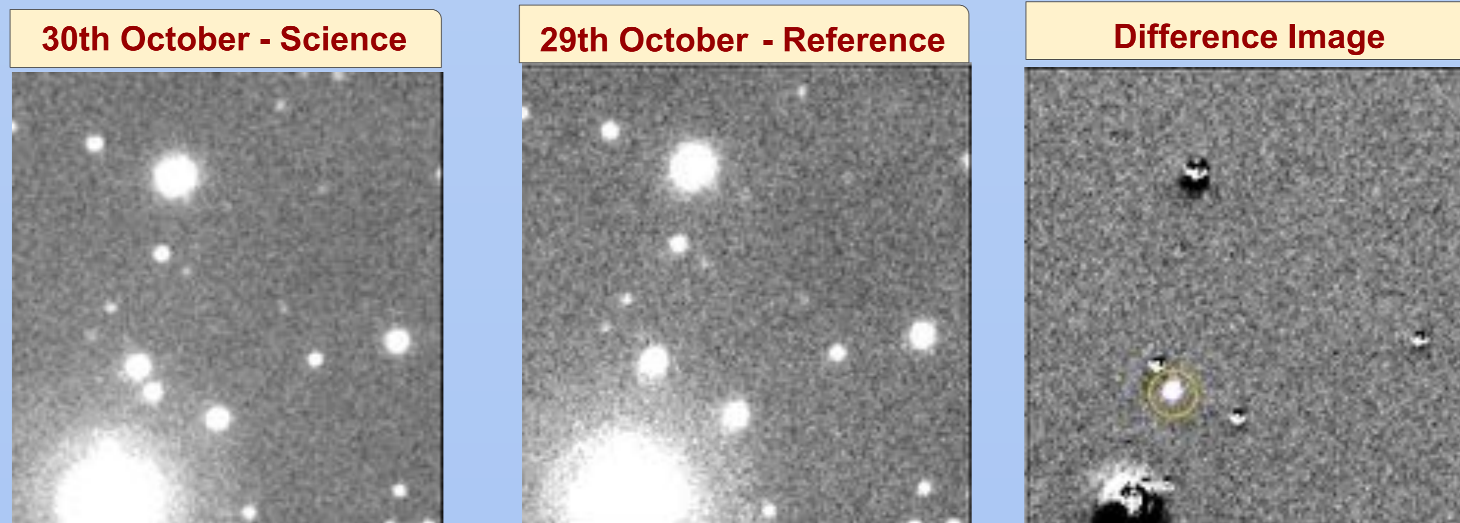
Fig. 2: Figure illustrating science, reference and difference image of the same region of the sky falling in the ILMT field taken in i band. The science image was taken on 30th October at 4h 31m LST while the reference image was taken on the previous day at the same sidereal time. The CNN based real/bogus classifier successfully identified an asteroid candidate in a region of the field in the difference image which has been highlighted using a golden circle.
