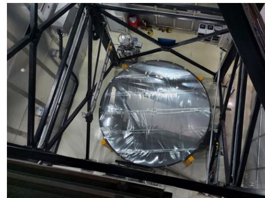
Fig. 3: Top view of the ILMT structure and mirror filled with mercury and covered with mylar
